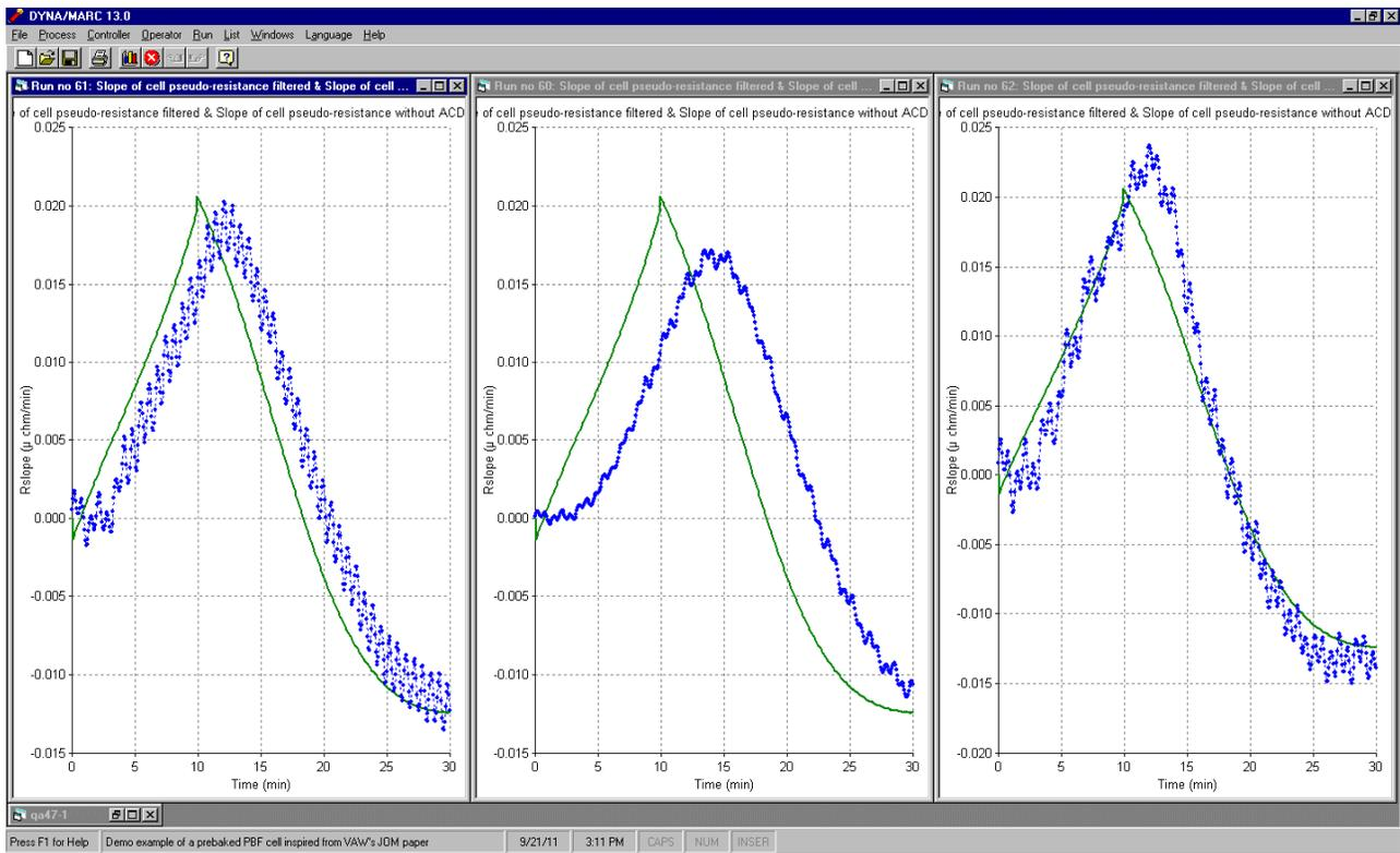
Figure 2: Noise-free (in green) and filtrated (in blue) slope of the cell pseudo-resistance using 60 datapoints linear RMS fit on the left, 120 datapoints linear RMS fit in the middle and 120 datapoints quatratic RMS fit on the right.
