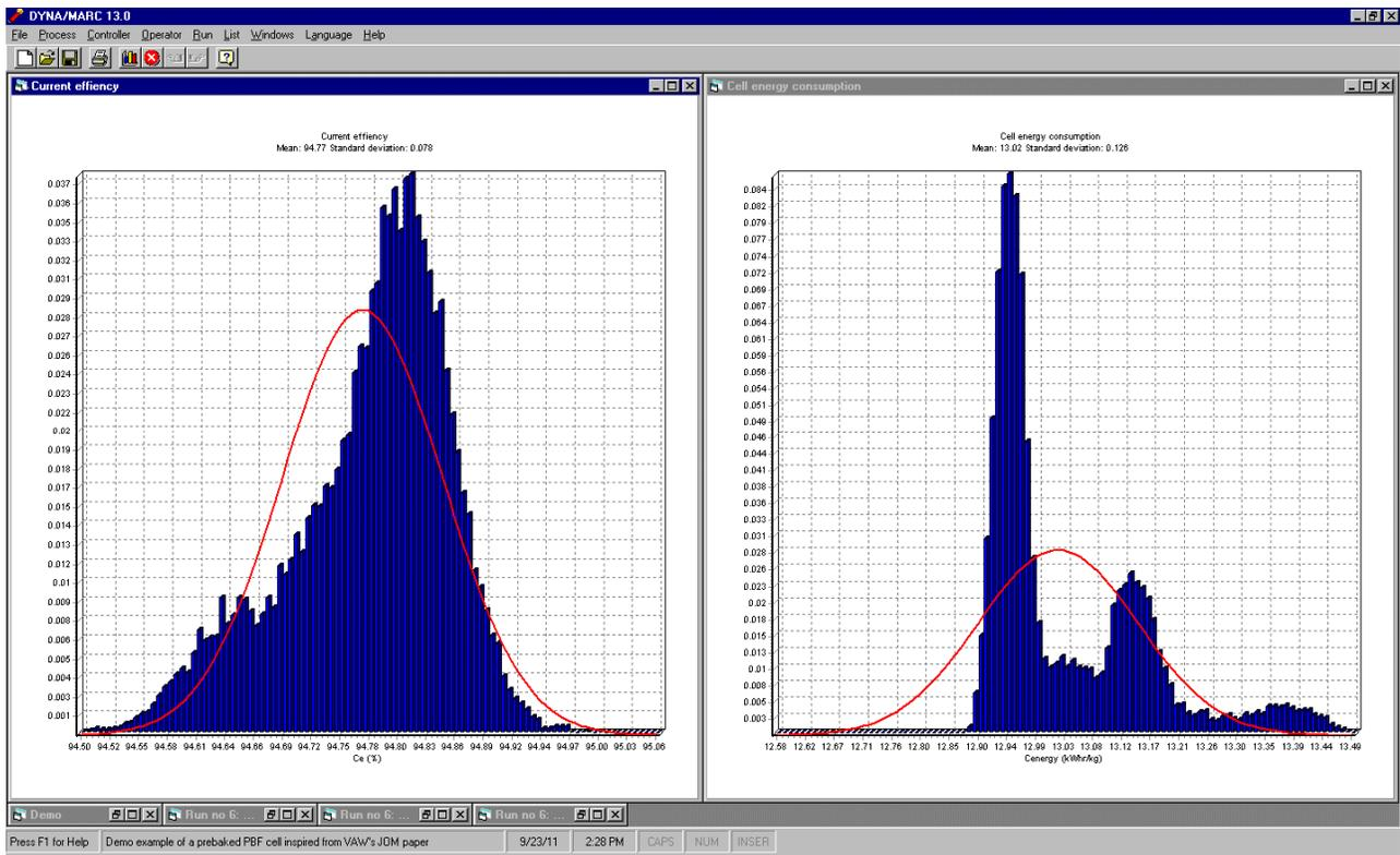
Figure 14: Predicted 24 hours averaged cell power and current efficiency, using the *In Situ* Feed Control
