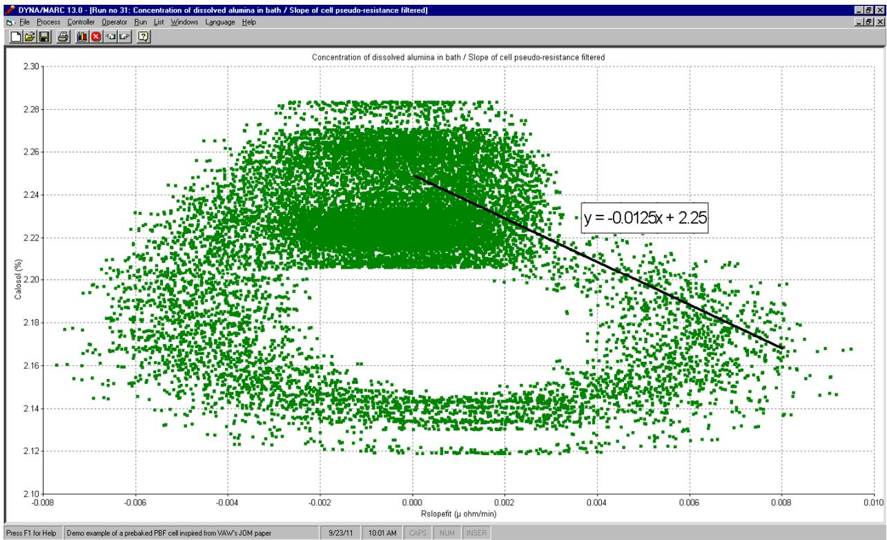
Figure 12: Correlation between the slope of the normalized cell voltage and the dissolved alumina concentration for that 24 hours simulation
