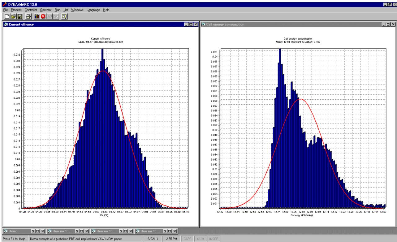
Figure 8: Predicted 24 hours averaged cell power and current efficiency, using the Demand Tracking Feed Control
