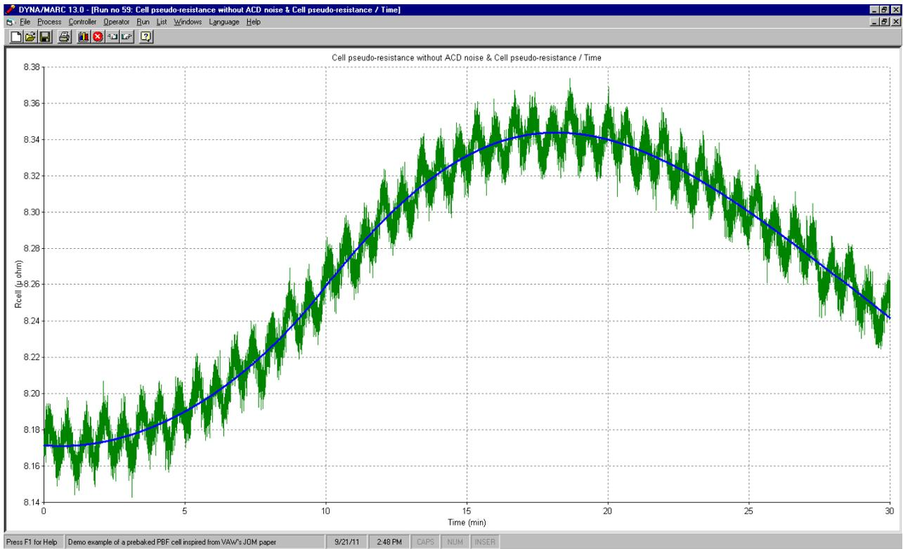
Figure 1: Noise-free (in blue) and noisy (in green) cell pseudo-resistance evolution as generated by Dyna/Marc cell simulator
