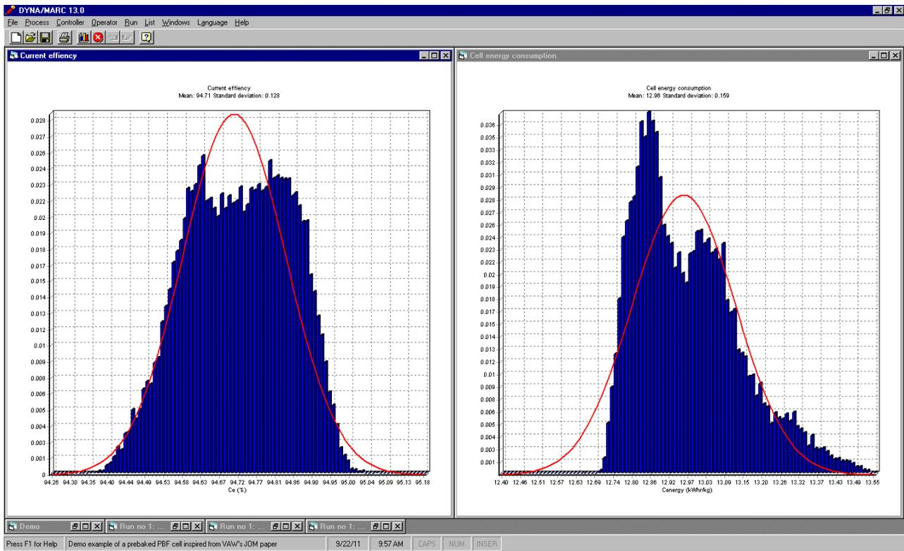
Figure 4: Predicted 24 hours averaged cell power and current efficiency, using the Pechiney Tracking Feed Control
